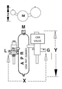
The APR Control Compressor Ratio Reduction Valve should be set to begin opening at approximately 60 PSI ~34°F
